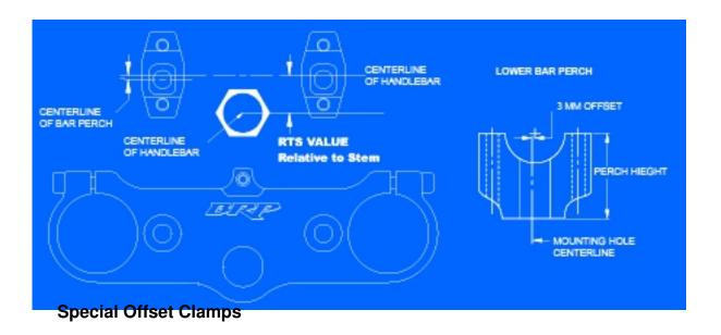
What is a triple clamp offset? Triple clamp offset is the distance measured between the centerline of the
